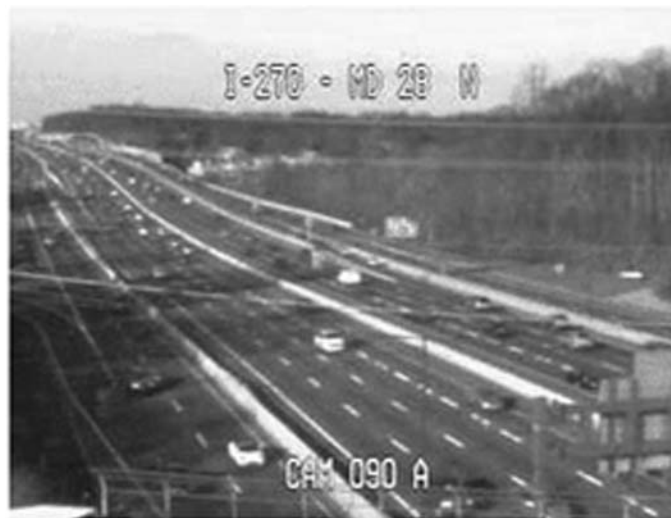
Figure 6-3. Traffic Camera Can Also Generate Flow Data.
